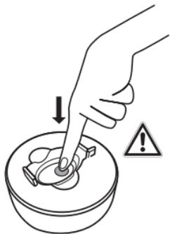
If pressure has built up in the food jar, you can relieve it carefully by pressing the pressure relief valve.
