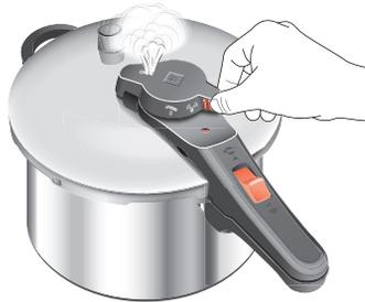
Abb. 17: Fast pressure release
