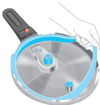
Abb. 6: Afdichtring lostrekken
