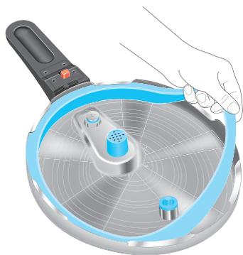
Abb. 6: Detaching the sealing ring
